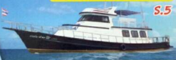
LENGTH 17.0 M BREADTH 4 M TWIN ENGINE DIESEL 185 HP
