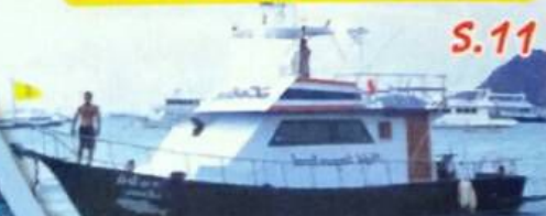
LENGTH 17.0 M BREADTH 4 M TWIN ENGINE DIESEL 185 HP
