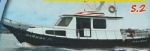
LENGTH 14.0 M BREADTH 3.2 M ENGINE DIESEL 185 HP
